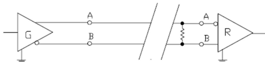
Figure 51-2: Termination differential input
