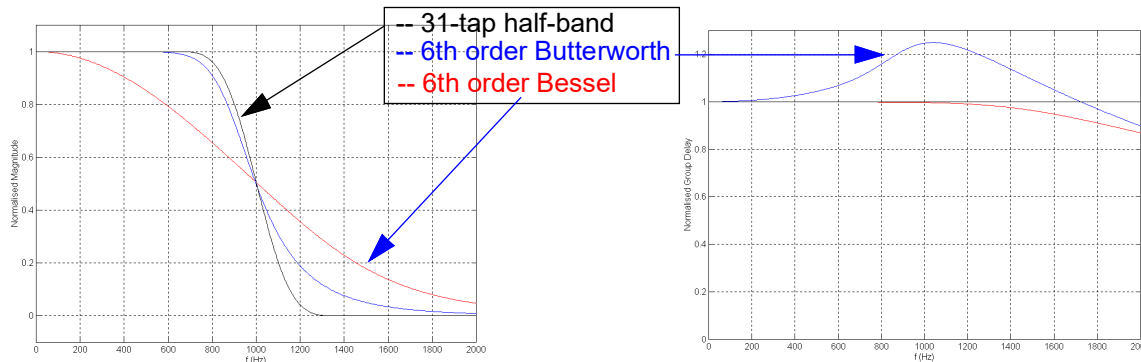
Figure 14-10: Normalized amplitude response and group delay for a 6th order Butterworth, Bessel and a 31-tap half-band filter
