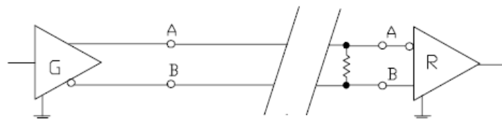
Figure 35-2: Termination differential input
