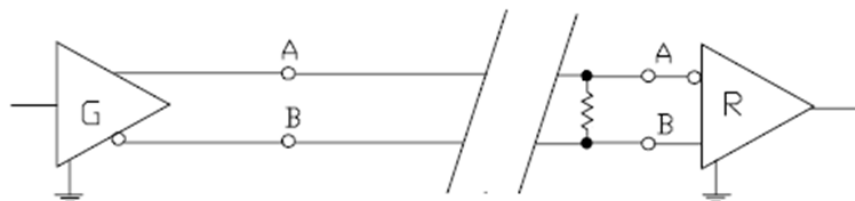
Figure 51-2: Termination differential input
