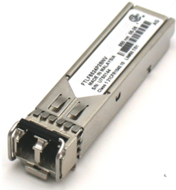
Figure 4-3 Pluggable (SFP small form factor)
