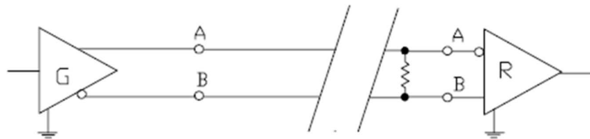
Figure 51-2: Termination differential input
